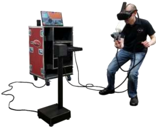
SimSpray console and user wearing the VR headset and the specially adapted spray gun
